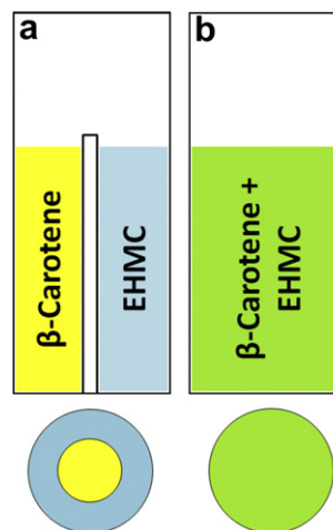
Fig. 2. (a) Core/shell configuration of \beta -carotene and 2-ethylhexyl 4-methoxycinnamate in tandem cuvette cell. (b) Homogenous configuration of \beta -carotene solution and 2-ethylhexyl 4-methoxycinnamate in standard cell.
